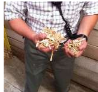
SCRAP WOOD FROM THE FACILITY'S PALLET RECYCLING OPERATION IS SHREDDED AND FED INTO THE BIOMASS BOILER, WHICH PROVIDES HEAT TO THE ENTIRE FACILITY THROUGHOUT THE YEAR.
